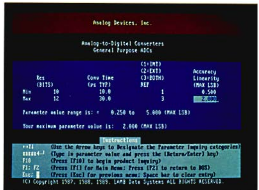
Figure 3. Screen for user entry of minimum and maximum performance parameters for general purpose a/d converters.
